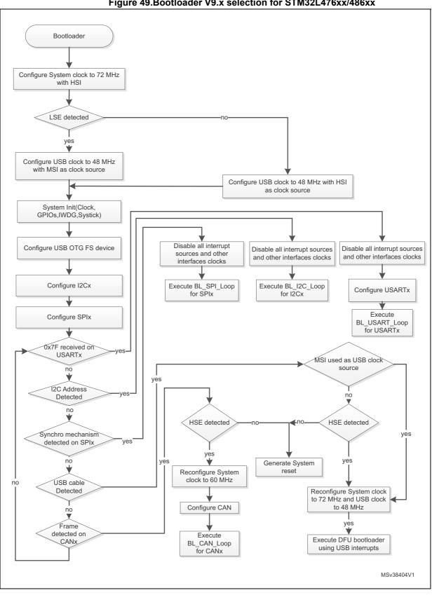
Figure 49.Bootloader V9.x selection for STM32L476xx/486xx
