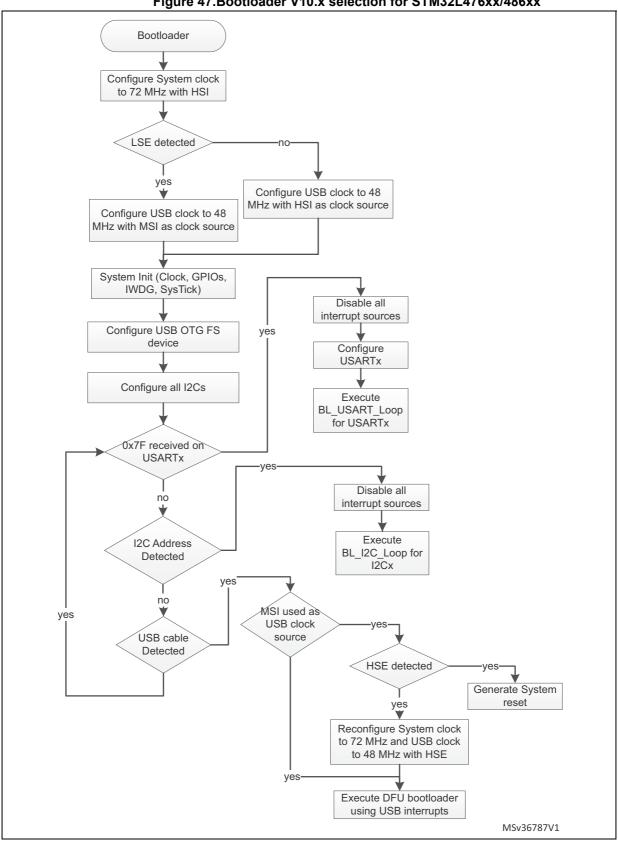
Figure 47.Bootloader V10.x selection for STM32L476xx/486xx
